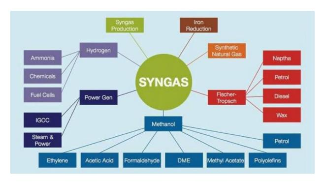
The primary products from plasma gasification are two: synthetic gas ("syngas"), and slag/vitrified glassy rock. Both of these products have high value, with syngas being the primary product. See attached chart of what syngas can be converted to. Depending on the regional economics, syngas can be used for electrical power, methanol or liquid fuels such as jet fuel, diesel, synthetic natural gas generation and others.
